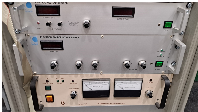
Figure 3: The Electron Source Power Supply (middle) and Glassman WR series HV supply (lower)
