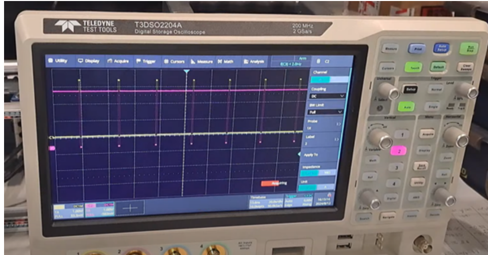
Figure 14: Oscilloscope reading for the digital outputs from the valve program
